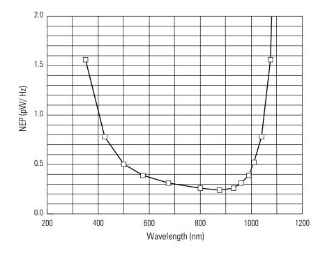
NEP as a function of wavelength for Model 2011 (at 10<sup>4</sup> Gain Setting).
